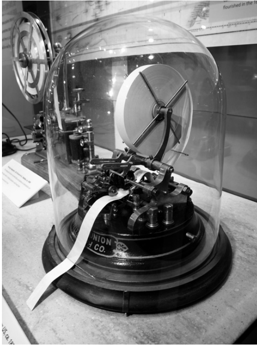
FIGURE 3.1 Western Union Ticker Model 3-A. WU first introduced its popular stock ticker in 1866. The Universal Model 3-A ticker was designed by Thomas A. Edison in 1873 and sold through about 1900. Credit Don DeBold, licensed under CC0-1.0.
